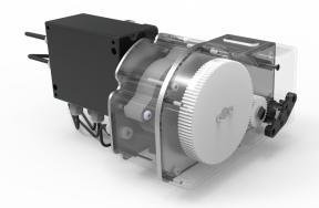
The **BARO Drive by Wire** system provides an ARM Cortex M4F processor running at 120 MHz that offers a powerful speed to process all the commands received from the main computer to move the steering wheel.
